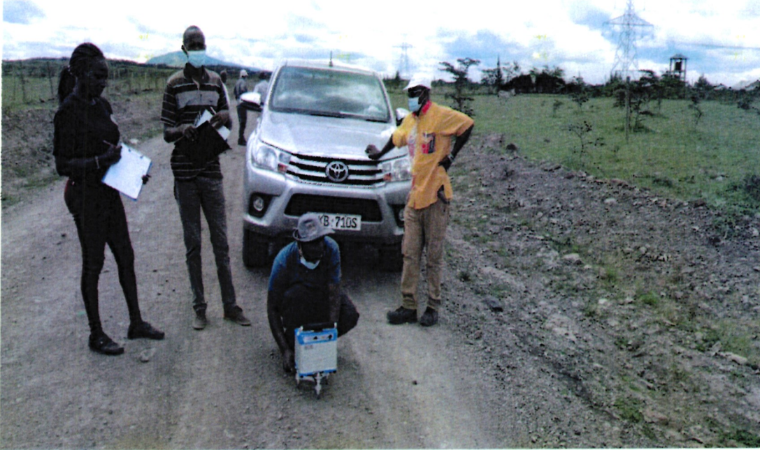
Gravity data acquisition of the Kipetu Gas Prospect, Kajiado County
