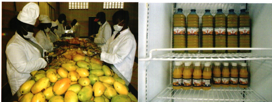
Production line: peeling, pulping, pasteurization and cooling of mango pulp, at Malindi Pilot Plant (left) and bottled fresh mango juice stored in a fridge (right).
