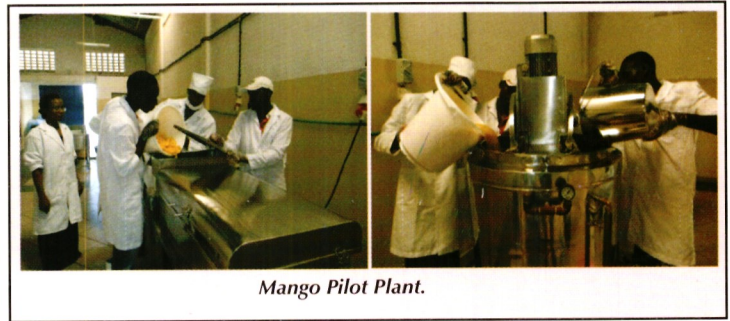
Testing of the fruit pulper (left) and pasteurizer (right) at Malindi
