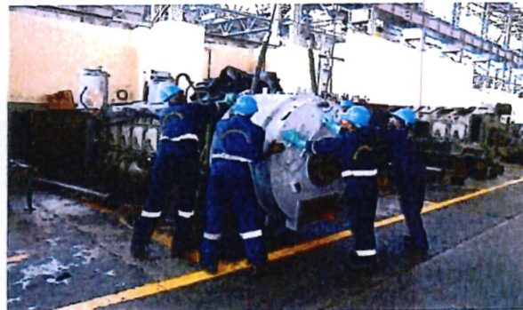
4 X Locomotives Class 93 rebuilding of engines
