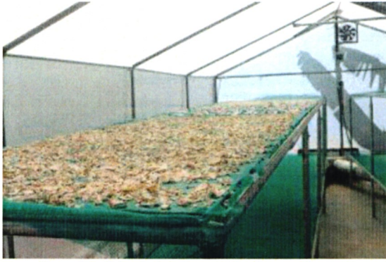
Sample of the Solar Dryer Machine to be developed by the Agriculture Engineers at JKUAT
