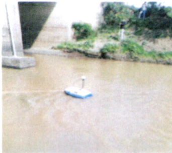
Discharge and Velocity Measurements for The Purpose of Calibrating the Sensors
