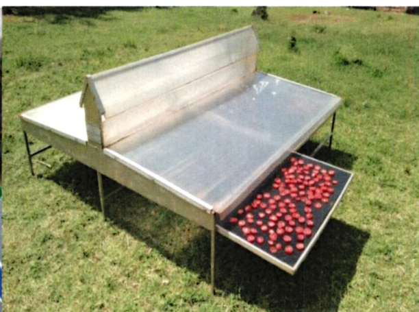
Tapros Solar Dryer developed by Homa bay ATDC
