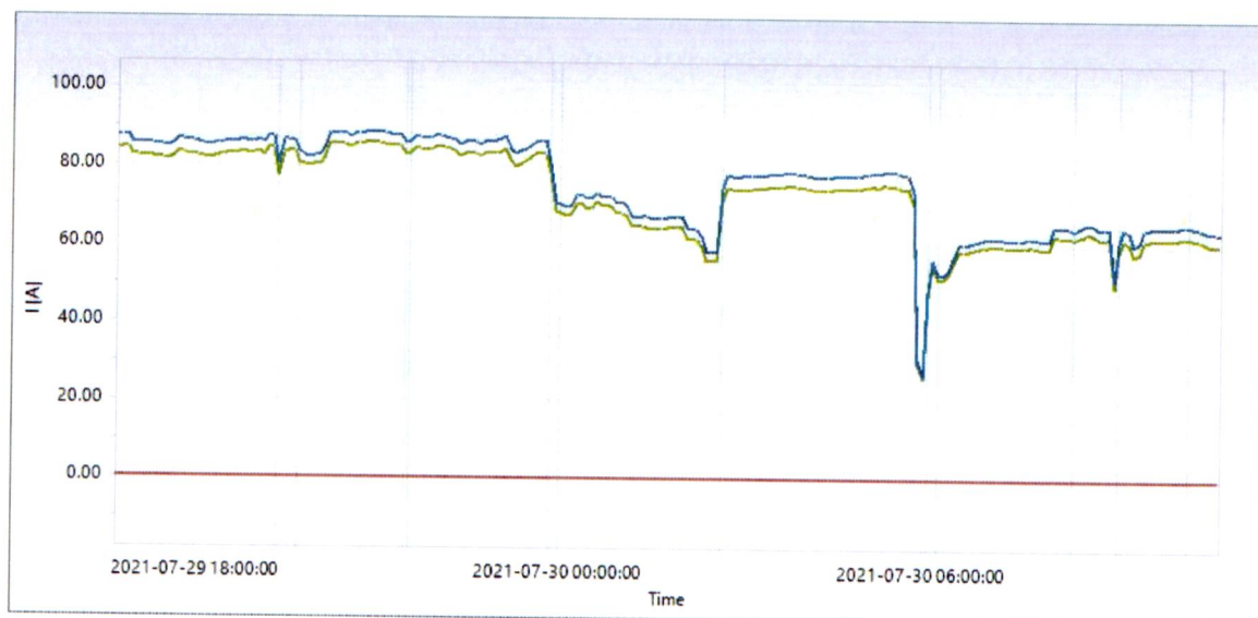
A logging of Currents at the 33kV metering point
