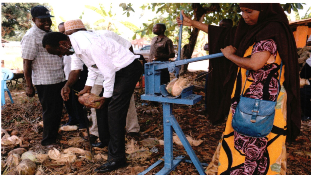
Prof. Ikua (left) tries to dehusk using a crude equipment, while (right), a member of Msambweni Coconut Producers performs the same task using the new dehusker.
