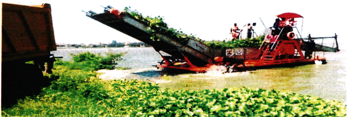
Picture 9: Test run of the water hyacinth harvester procured by LVEMP II Kenya for mechanical removal of the weed
