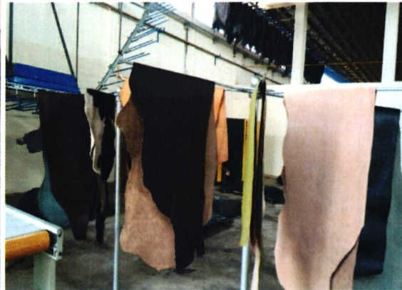
Installed overhead dryer
