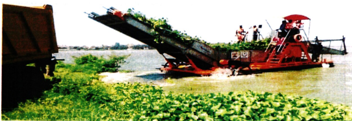
Picture 9: Test run of the water hyacinth harvester procured by LVEMP II Kenya for mechanical removal of the weed
