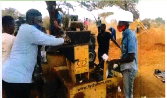
Youth making soil blocks using ISSB technology that will be used to construct 30 additional classrooms at Mikuyuni Secondary School in Kibwezi .
